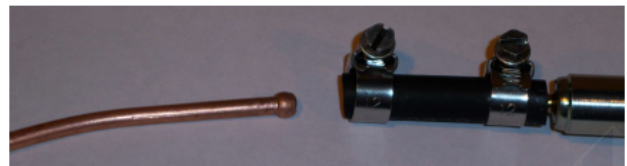
Flared end of copper pipe
